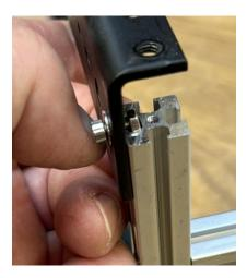
• Insert a support beam *underneath* the short leg of the rack post. Attach the beam to the side beam (and rack rail) using a M3 washer and M3x**25**mm screw.
